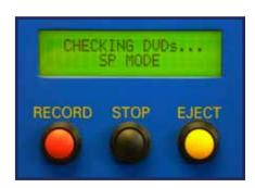
5. WAIT UNTIL THE ALARM SOUNDS WITH THE MESSAGE "READY TO RECORD", THEN PRESS THE RECORD BUTTON: THE EQUIPMENT WILL NOW START RECORDING.
