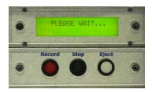
When the LCD message display shows the following message: "PRESS EJECT TO INSERT NEW DVDs" then the AVN 200 Portable DVD Interview Recorder is ready to be used.
