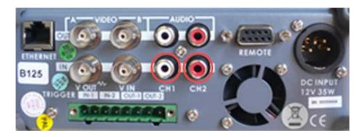
vi. Connect black "D type" cable (9 pin connector) to 9 pin socket at the rear of the AVN 200 Portable DVD Interview Recorder. Then connect the remaining end to the "Remote" socket at the rear of the hard drive.
