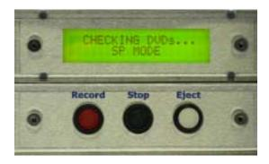
4. WAIT UNTIL THE ALARM SOUNDS WITH THE MESSAGE "READY TO RECORD", THEN PRESS THE RECORD BUTTON: THE EQUIPMENT WILL NOW START RECORDING.
